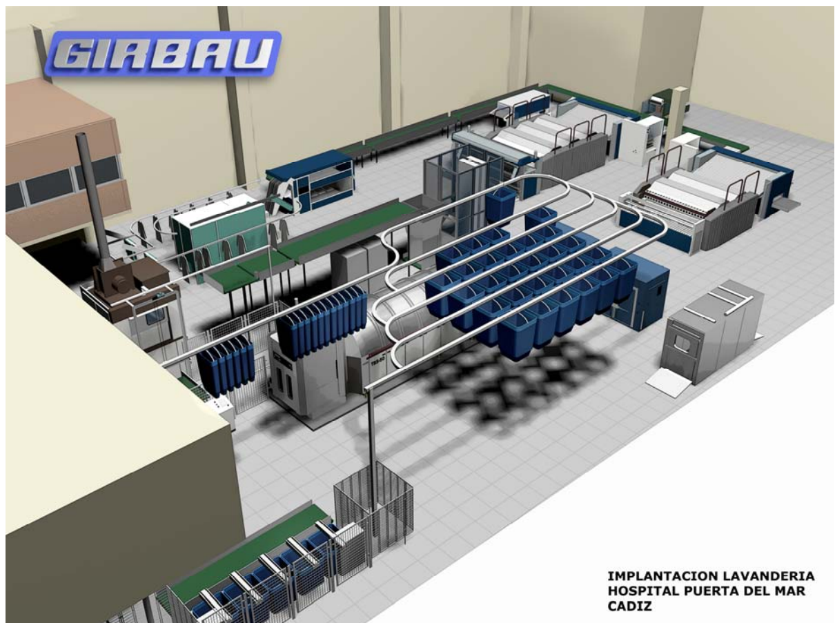
A monorail loading system transports the bags of dirty linen direct to the batch-washer
