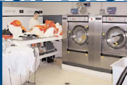
Sevier County's two 55-pound, soft-mount Continental Pro-Series™ Washer-Extractors and two 75-pound dryers have boosted the facility's production and slashed utilities.
