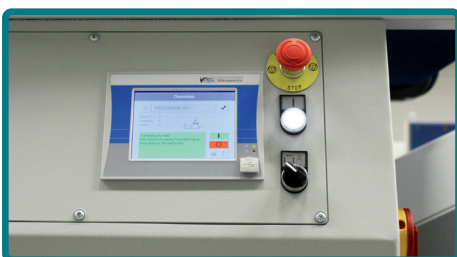
Touch screen PLC control
