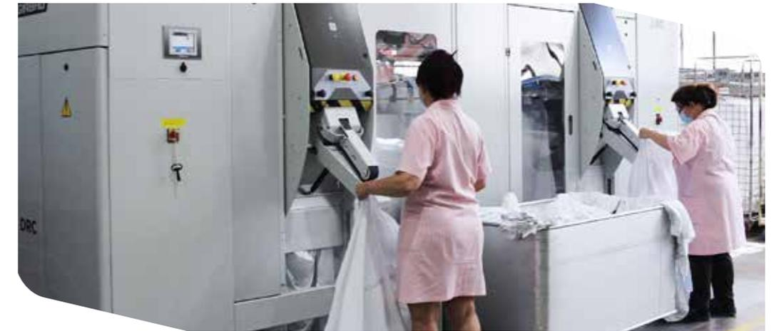
This year we have completed the project for the first cornerless feeder, the DRC, which allows textiles to be fed in without the need to find the corners.
