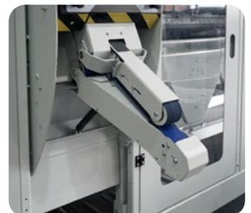
Cornerless feeder for any high-speed ironing train. One, two or three-station feeder for fast feeding of single sheets like hospital bed linen.
