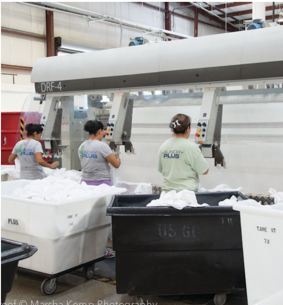
Operators clip sheets onto DRF feeder.
