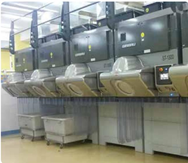
of small items using the PC120 flatwork ironer. The ergonomics of the work positions, with their adjustable height, make it easier to feed linen and improve the productivity of the operators in the process.
