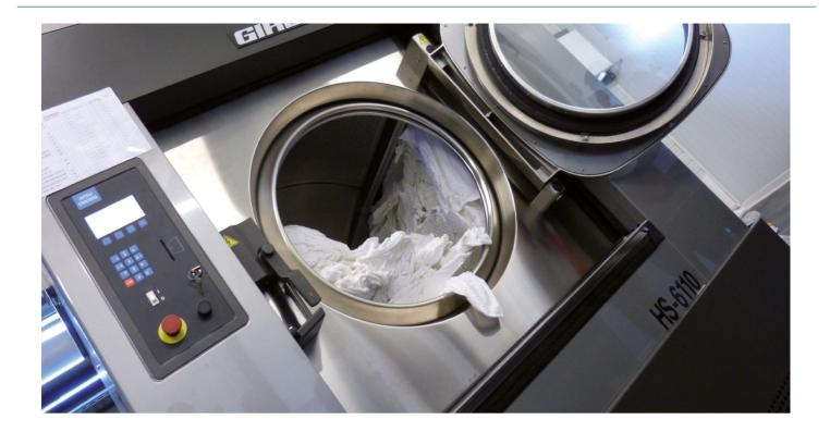
HS high-speed washing machines allow high output and give the business flexibility by enabling it to adapt water levels to the actual load volume, substantially reducing consumption of water and detergents, so benefiting the company's operating account.
