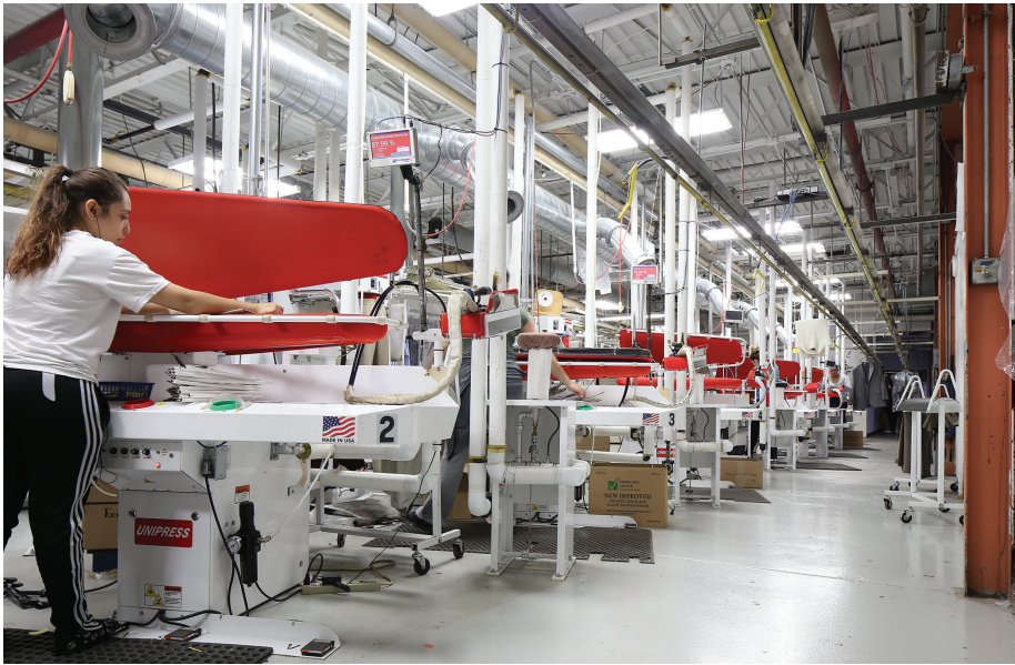
Eight Unipress pant-pressing stations have cut labor hours and boosted throughput and quality.
