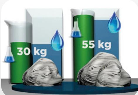
**Proportional load:** The dosage of chemicals and water is automatically adjusted depending on the load, which can range from 30 to 55 kg.
